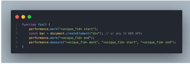
Figure 3: Example of inserted performance marks
