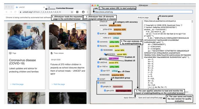
Figure 1: JSAnalyze User Interface: From entering a URL to generating a simplified page for mobile web.
