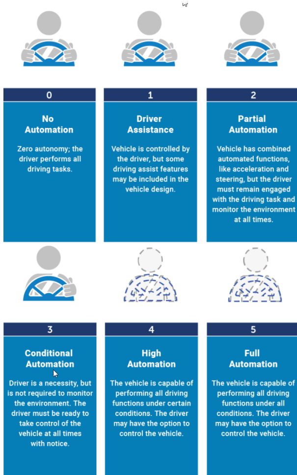
Figure 1: Levels of Vehicle Automation [4]
