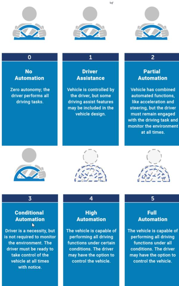
**Figure 1: Levels of Vehicle Automation**
